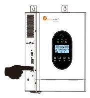
Once the unit has been properly installed and the batteries are connected well, simply press On/Off switch(located on the Left sideof the case) to turn on the unit.
